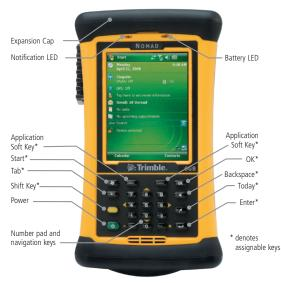
NOTE: If your unit has the following features, these keys are assigned: Flashlight - Left Softkey; Scanner - Right Softkey; Camera - Today Key
